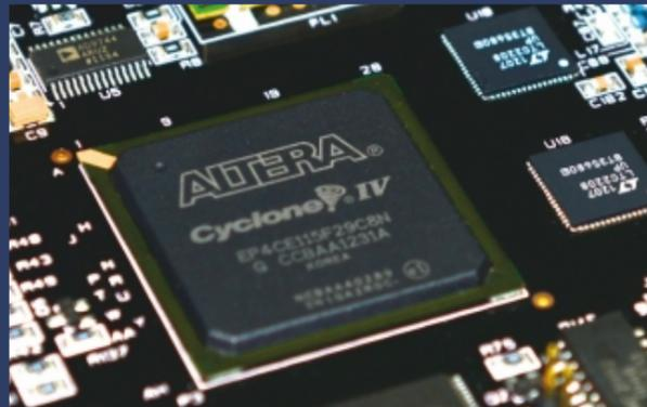
The ANAN-100D/200D have true phase coherent dual front end comprising of two 16 bit 130MSPS ADCs and a large Cyclone IV FPGA which allows for a huge amount of headroom and DSP processing power, the current firmware incorporating 14 receivers and diversity reception uses around 30% of the FPGA resources!
