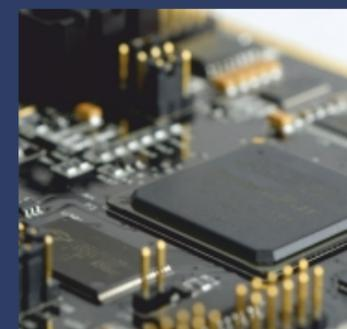
Highly integrated 8 layer design, use of state-of-the-art FPGAs enables huge DSP processing capability and logic implementation.
